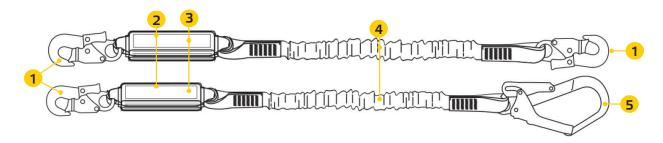
The Energy absorber is made of 32 mm wide webbing. The absorber is equipped with attachment loops on the endings which are integrated with a lanyard. The body of the absorber is protected by a special jacket made of a shrinkable, polyethylene tube. The lanyard is made of 30mm wide polyamide webbing. The endings of the lanyard are sewn making the attachment loops.
