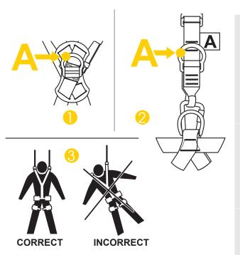
**Fall arrest system** must be connected only to the attaching elements of the harness marked by capital letter A. The fall arrest system must be connected only to: - dorsal attachment D-ring - drawing (1) or - to frontal attachment D-ring. The dorsal attachment D-ring is marked by a capital letter A - embossed on the crossing plate. Front attachment D-ring is marked by a capital letter A placed on the label sewn near the D-ring . See drawings 1 and 2.
