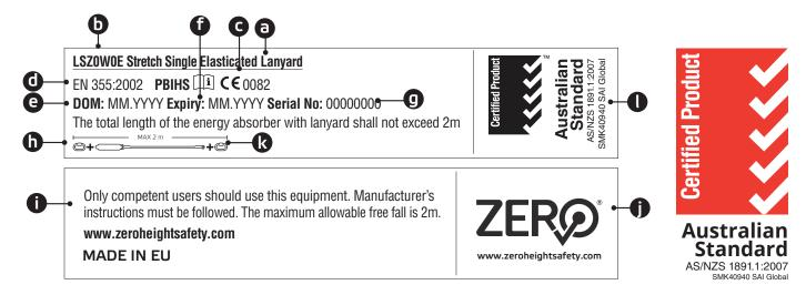
> Make sure that all labels on protective equipment (elements of this equipment) are legible while performing a periodical inspection.
