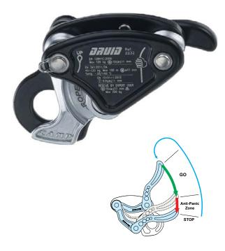
A lightweight, compact auto-braking descender for rope access and rescue designed for semi-static ropes ranging from 10-11 mm. Designed with an anti-panic function the body and lever are made of robust hot-forged aluminium alloy. The internal mechanism and locking cam use a patented design for smooth action on the rope which prevents rapid wear-and-tear and absorbs energy from small shocks with a slight amount of rope slippage.
