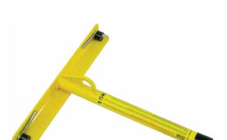
A Simple and effective primary anchor for access onto sheet metal roofs, the ZERO® Anchor-to-Go has interlocking cam clamps to secure the anchor to the edge of the roof sheeting (in the gutter line). This fast setup makes the Anchor-to-Go perfect for plumbers, painters, service technicians and installer that require short term roof access.
